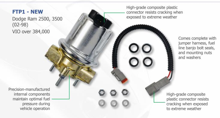
**Tech Tip:** Fuel transfer pump pressure should be 8-10 PSI during cranking and more than 5 PSI during vehicle operation.
