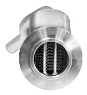
**OE Design:** Fin-and-tube **Effect:** Although this design is efficient, it's prone to soot clogging and internal leaks from fractures caused by overheating
